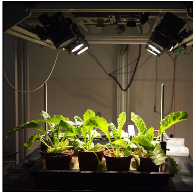
Fig. 3. Reference HSI camera assembly on gantry, showing ImSpector (top centre left) camera and halogen light sources
