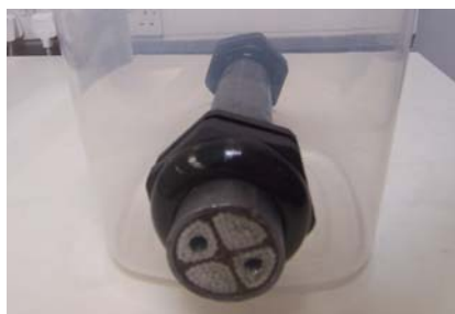
Figure 9. Full cable sample. Holes seen in two of the conductors are for heaters; there are also two at the other end of the other two conductors.
