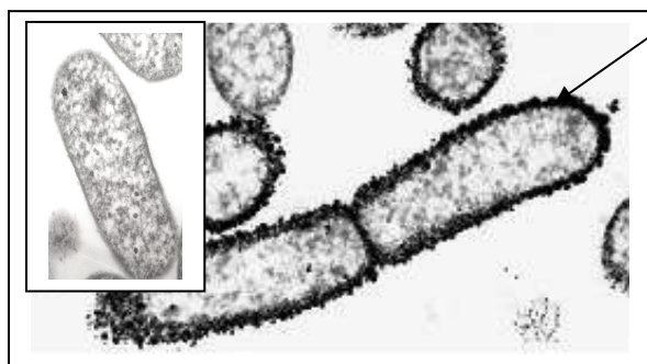
Fig. 2. Palladized cells of Desulfovibrio desulfuricans . A non-palladized cell is also shown (inset). Palladization involves pre-incubation with Pd(II) to saturate biosorption sites, followed by addition of H 2 to achieve reduction of Pd(II) to Pd(0) via hydrogen-ase [13]. Particle growth to the correct size is achieved via autocatalysis via the Pd nanoclusters; cellular viability is not required after the initial nucleation. The laboratory ‘workhorse’ Escherichia coli and other bacterial strains can be similarly used to make catalysts with similar catalytic activities.
