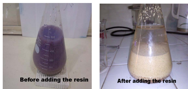
Figure 1. Photo shows ion exchanging before and after adding the clean resin to the solution of cesium and cobalt.
