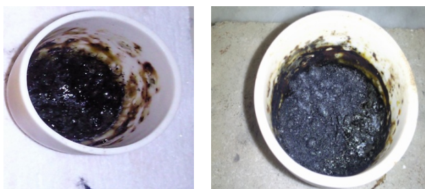
Figure 10. Photo shows the final glass matrix from the first batch bearing high content of sulfur.
