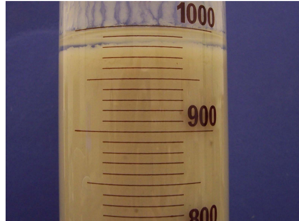
Figure 7 Bleed test result - 5-min hydration and 5.0 g/L de-icer
