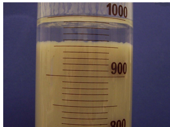
Figure 8 Bleed test result - 5-min hydration and 7.5 g/L de-icer
