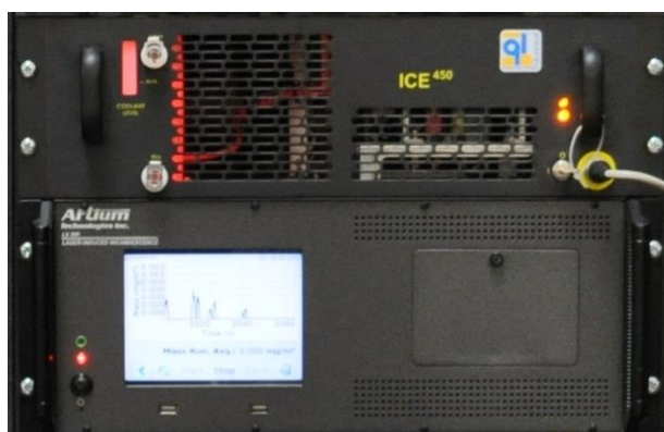
Figure 18 Artium LII-300 and AVL MSS nvPM mass instruments
