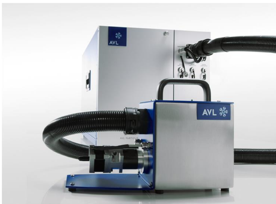
Figure 17 Photograph of commercially available VPR incorporating a catalytic stripper
