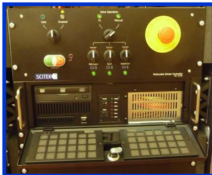
Figure 21 Photograph of 3PTS Control and Data Acquisition system
