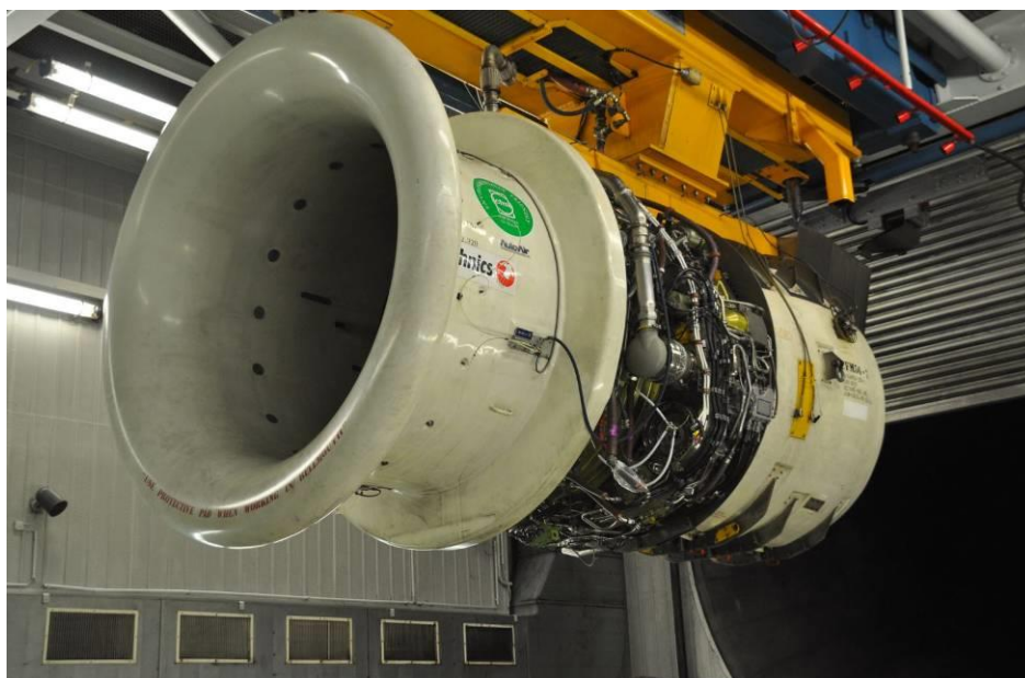
Figure 39 CFM56-7B26/3 mounted in SR Technics test Cell
