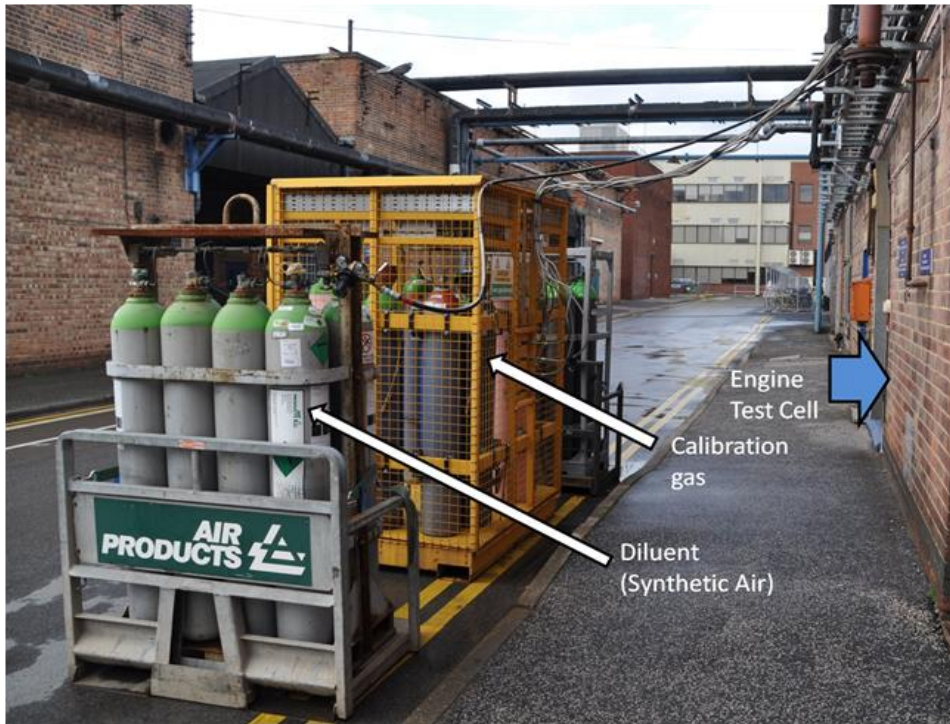
Figure 100 Setup of diluent and calibration gas bottles for Gnome engine testing
