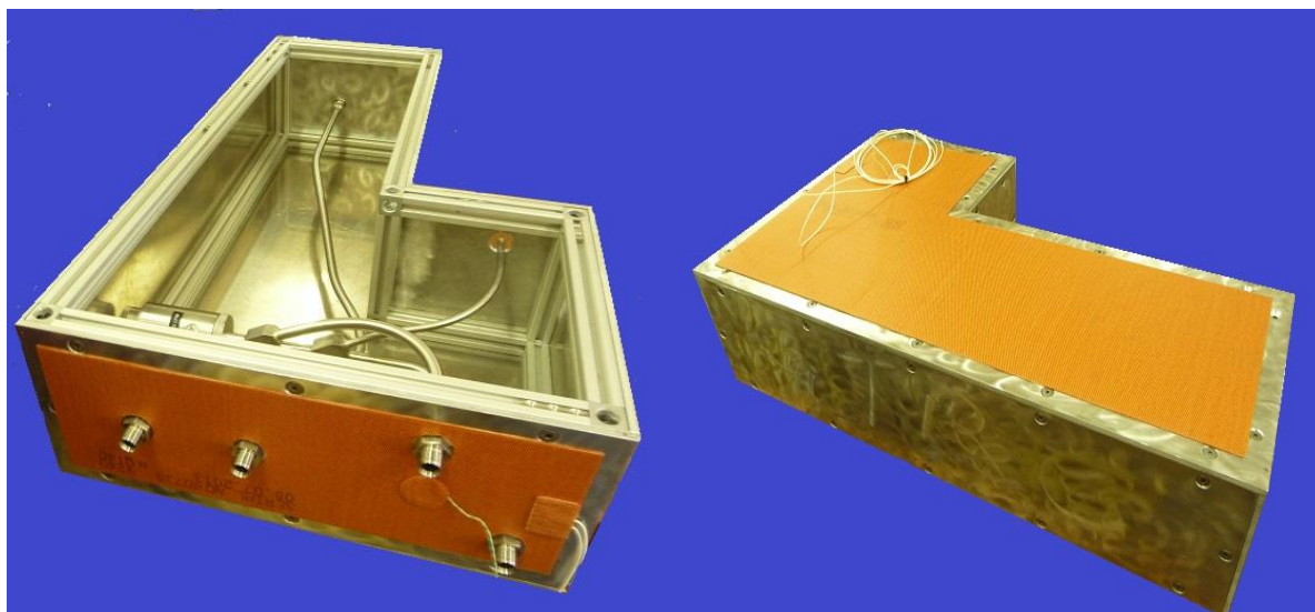
Figure 16 (a&b) Bulkhead and top heating mats of cyclone and secondary splitter oven (5PTS)
