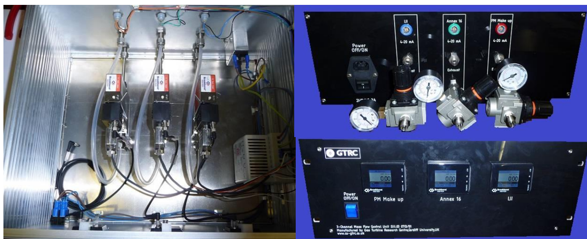
Figure 19 Photographs of Internal setup, back panel and front panel of 3 channel MFC control unit
