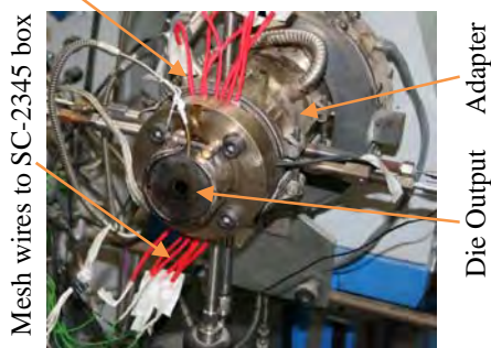
Fig. 1: Extruder die, adapter, & TC mesh
