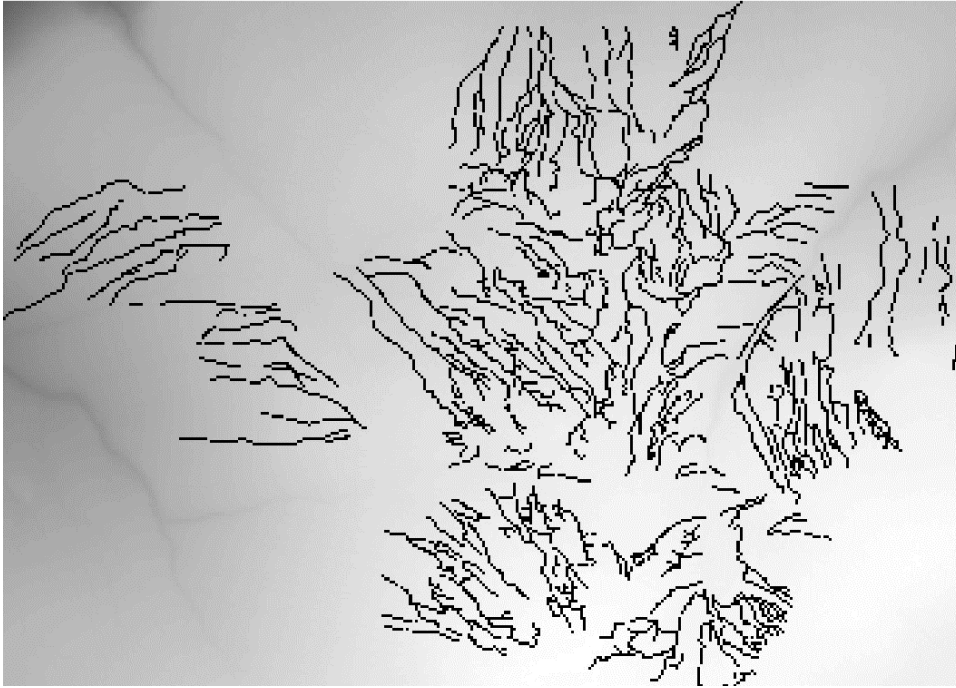
Figure 4.10 DTM with digitised gullies shown in black for a small part of the study area
