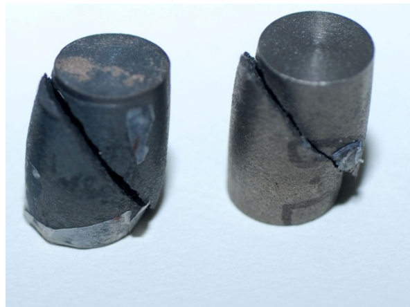
Figure 12: a) Ambient temperature stress-strain diagrams of cast iron (Group F and H tests) and b) shear failure mode of Group H specimens.
