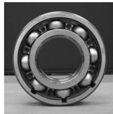
Fig. 14 Artificial bearing fault for fault severity analysis
