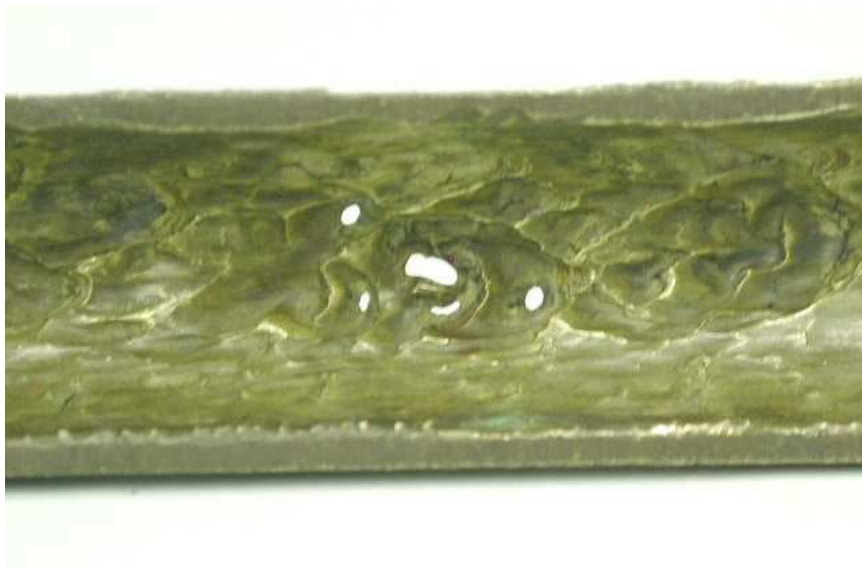
Figure 1: Surface stress corrosion cracks initiating from a pit in 316L stainless steel exposed to a MgCl_2 salt deposit at a relative humidity of 30% and at 40°C.
