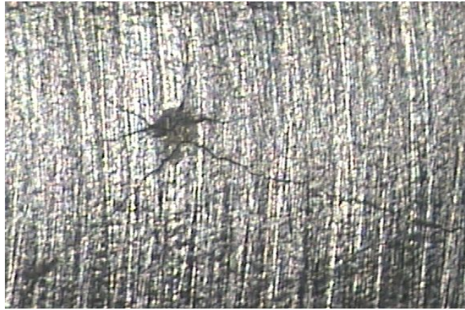
Figure 1: Surface stress corrosion cracks initiating from a pit in 316L stainless steel exposed to a MgCl_2 salt deposit at a relative humidity of 30% and at 40°C.
