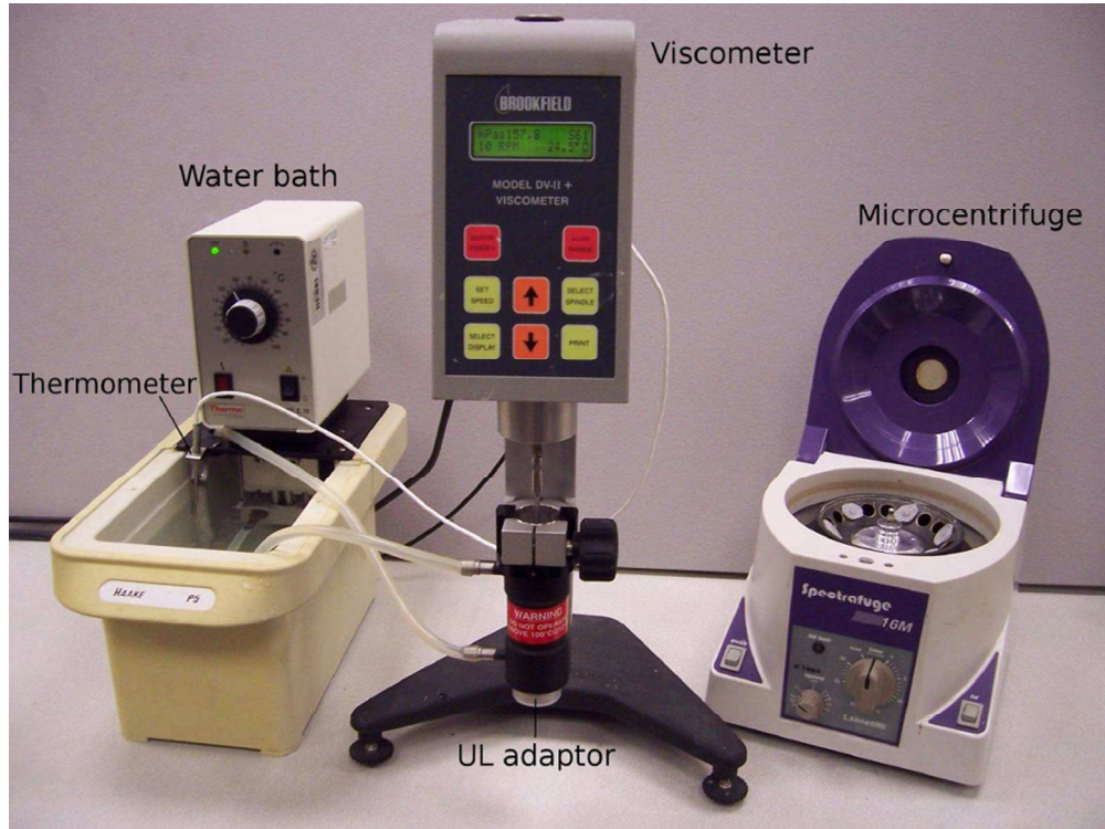
Equipment setup for the proposed viscosity method 85x63mm (300 x 300 DPI)
