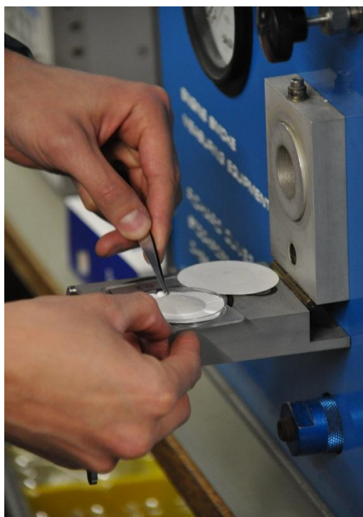
Figure 33 OCEC filter paper being removed from Smoke Number filter holder
