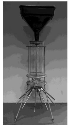
Figure 1. Cone splitter
