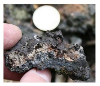
Figure 1 Gravel-size ash clinker particle with colourful bands (photograph taken at Northwich tipping site, Cheshire).
