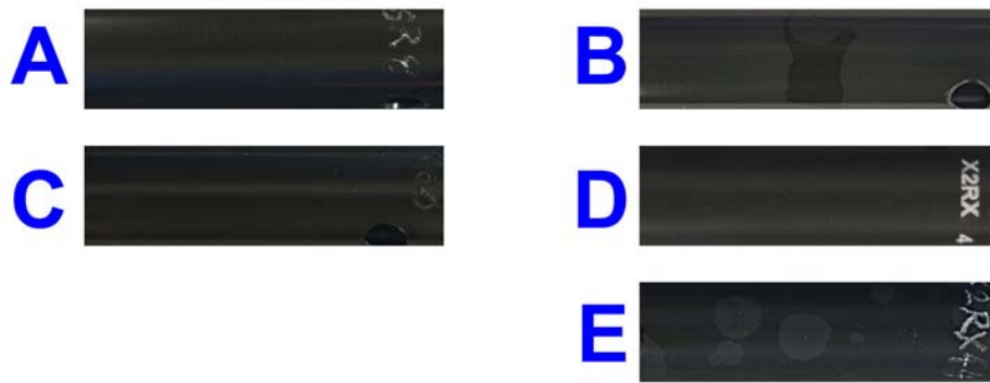
Figure 4: Autoclave corrosion weight gain profile of non-hydrated A-0.0Sn SR and RX materials. Photographs of actual corrosion specimens included: (A) non-hydrated A-0.0Sn – SR after 280 days of autoclave exposure, (B) non-hydrated A-0.0Sn – SR after 540 days, (C) non-hydrated A-0.0Sn – RX after 20 days, (D) non-hydrated A-0.0Sn – RX after 300 days and (E) non-hydrated A-0.0Sn – RX after 540 days of autoclave exposure.
