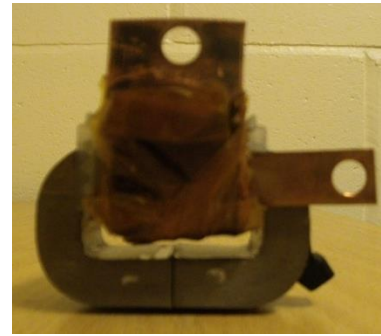
Figure A6.1: a) Dimension of AMCC-6.3 core (all dimensions in mm/mm 2 ) [54] and b) Photo of input inductor
