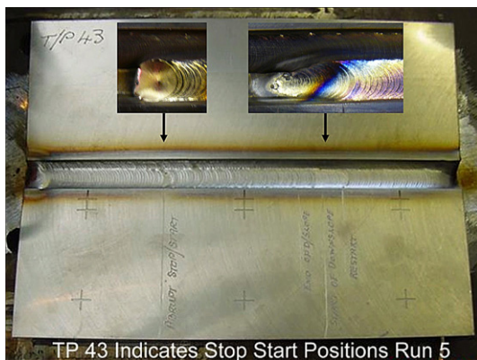
Fig. 2. Photograph of Plate 1 with fifth weld pass offset to one side of the groove (i.e. offset towards bottom of image). The welding direction was from right to left. Higher magnification images of ramped (right) and abrupt (left) interruptions are included as insets. The inset images were obtained from another test plate which was welded using the same nominal conditions. The weld pool was approximately 10 mm in length.
