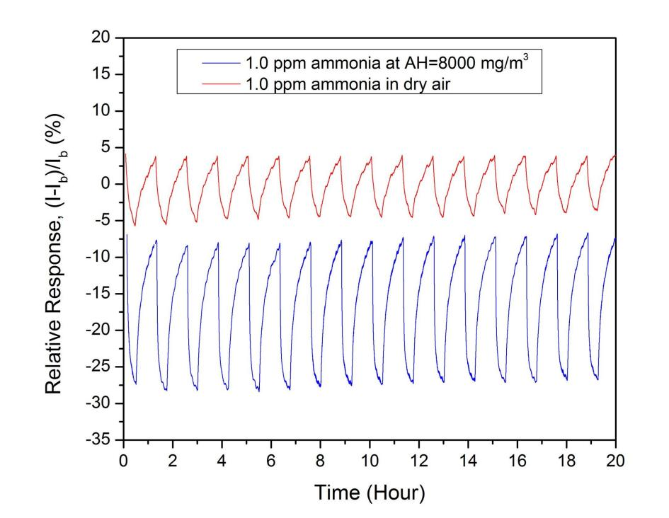
✓ Nafion-doped polyaniline sensor can be used as a humidity sensor as well. Water molecules ionise the terminal  $-SO_3H$  groups and increase proton conductivity. This increases the electrical conductance of the composite film.
