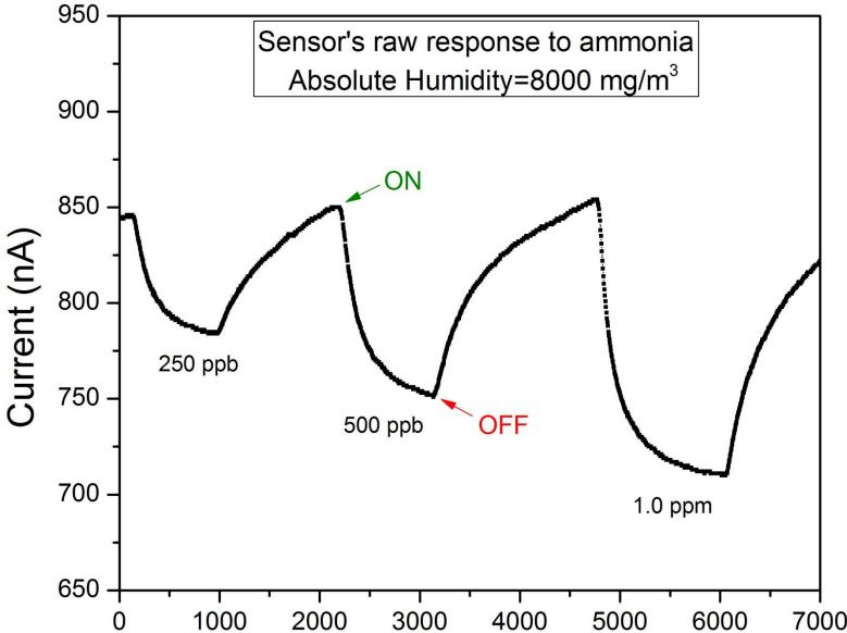
$\checkmark$  Repeatability test of the sensor to 1.0 ppm ammonia is shown. The sensor at humid environment works better.
