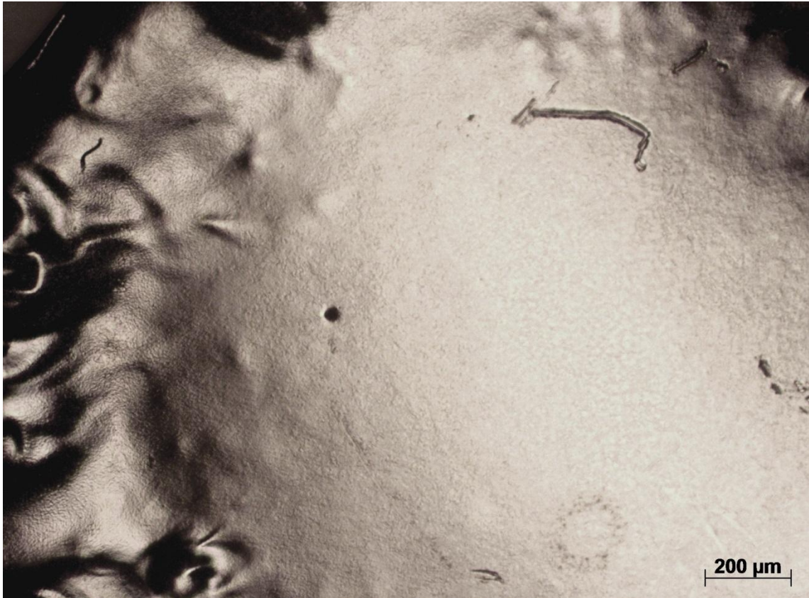
Figure 2: Light optical micrograph of the "electropolished" TEM-type specimen of weld P141 CAC S7
