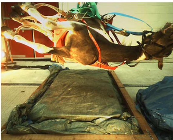
Fig. 3. Front view of Test 3 (side impact without ATD torso).
