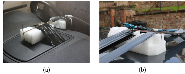
Fig. 2. The 1900 MHz dipole mounted on the (a) dashboard and (b) rooftop. Calibration standard used for in-situ VNA calibration can also be seen in (b).
