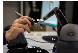
Figure 7: Phantom Omni device and the virtual vertical axis used in the audio-haptic design.
