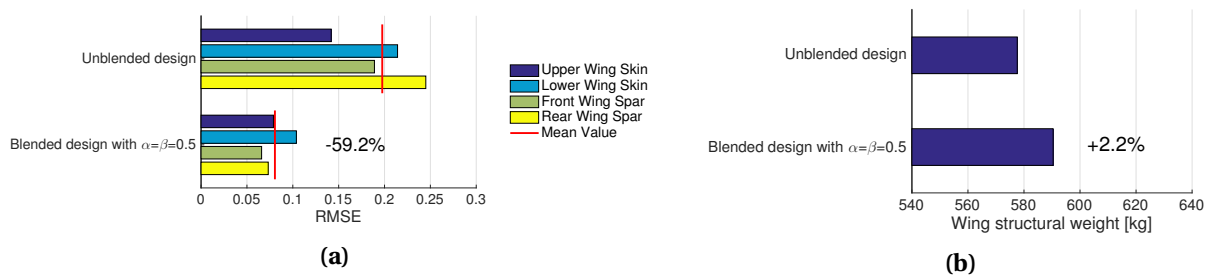
Figure 15: (a) RMSE in retrieving a blended structure, and (b) weight of the wing structure.
