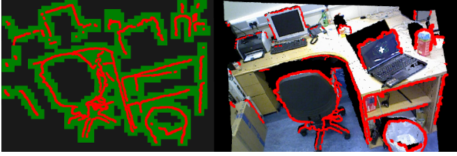
Fig. 2: Occluding depth edges (red) and the associated image patches which were flagged for edge detection (green).
