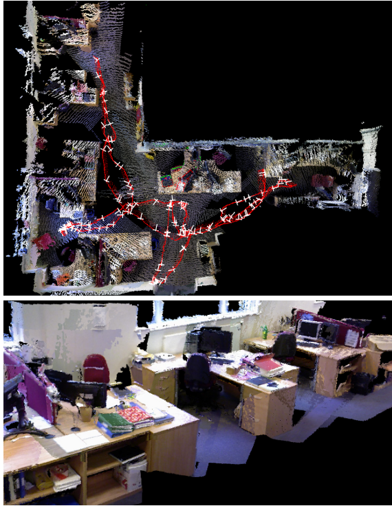
Fig. 4: An example map created by the proposed SLAM system. Key-frames poses are drawn in white and estimated camera trajectory (57m) in red.
