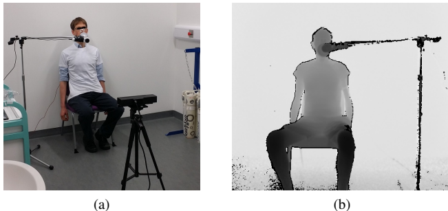
Fig. 13. (a) The proposed setup showing the Kinect in front and the spirometer mouthpiece (when used) on the subject, (b) A typical Kinect depth image.
