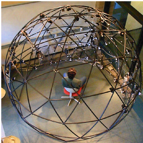
Figure 6: The mechanism used to generate the Yale Faces data set (Georghiades et al., 2001).
