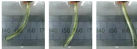
Fig. 3 Electrical actuation of biodegradable gelatine. Frames 4s apart.
