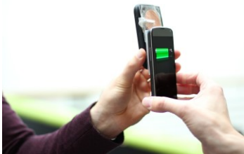
Figure 2: PowerShake prototype allows energy to be wirelessly moved between mobile devices, when in close proximity.
