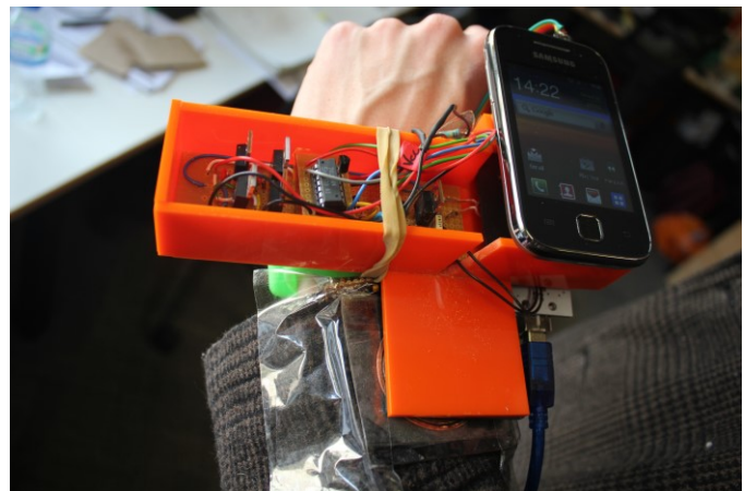
Fig. 13. Participant wearing the on-body garment power sharing distribution system, transferring power from the designated transmitter in the jacket pocket to the smartphone based on the wrist.
