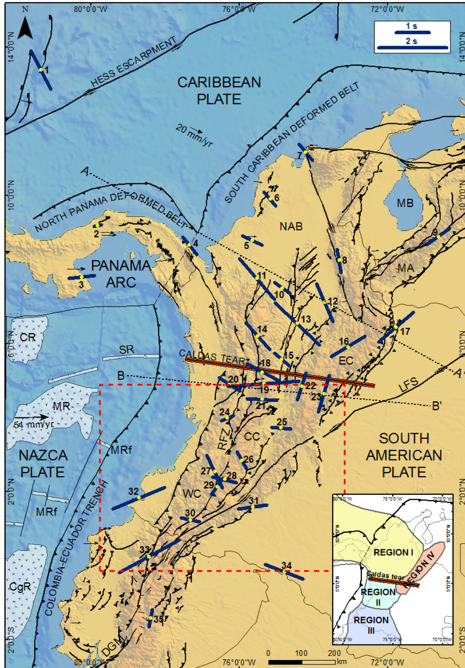
Figure 4. Stacked SKS shear wave splitting at each station (numbers correspond to those listed in Table 1). Orientation of the thin blue bars indicate fast component polarization direction ( \phi ) and the bar length is proportional to delay time ( \delta t ). Note the change in the dominant trend in \phi at \sim 5^\circ\text{N} (Regions I and II) and at \sim 2.8^\circ\text{N} (Regions II and III). Fast orientations also exhibit different trends at stations in Eastern Cordillera and Merida Andes (Region IV). Red box indicates the area shown in Figure 7. Profiles AA' and BB' are shown in Figure 9. NAB: North Andes Block; MB: Maracaibo Block; LFS: Llanos Fault System; DGM: Dolores-Guayaquil Megashear; RFZ: Romeral Fault Zone; MA: Merida Andes; WC: Western Cordillera; CC: Central Cordillera; EC: Eastern Cordillera; CR: Coiba Ridge; SR: Sandra Ridge; MR: Malpelo Ridge; MRf: Malpelo Rift; CgR: Carnegie Ridge. Inset map shows the four regions differentiated based on the SKS splitting behavior.
