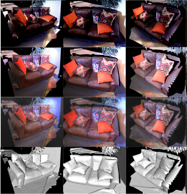
Fig. 10: Sofa. The LDR frames generated using [3] are shown in the first row and HDR frames produced by HDRFusion are shown in the second row and third row. The second row is generated using [8] where the colour saturation is set as 1. Comparing with raw RGB fusion [3], the dynamic range of the radiance texture is much higher. The details in dark area are well preserved. The third row is generated using [24], where the colour saturation is set as 1.25. [24] visualizes the rich details captured by HDRFusion. The bottom row shows the recovered surface geometry.
