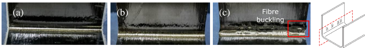
Figure 8 Internal corners of C-section preform produced by HDF process: (a) veil interleaved, (b) powder interleaved (c) non-interleaved.
