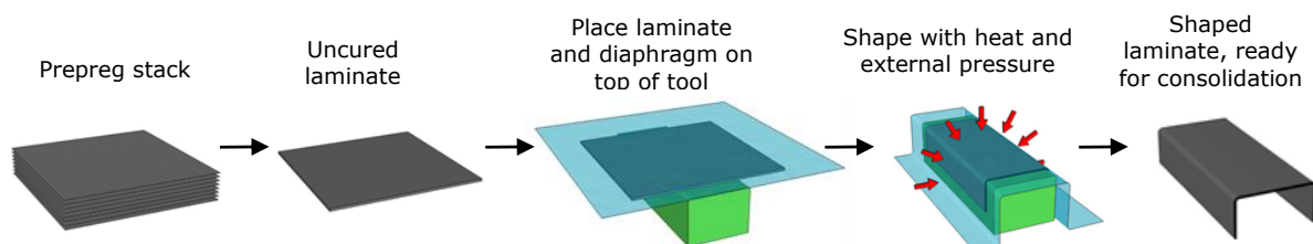
Figure 1. Illustration of composite vacuum forming process.
