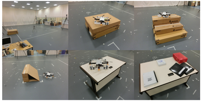
Fig. 2. Some of the obstacles used in the experiments. First row: the arena (also shows the RGB-D sensor on tripod), 'box', 'steps'. Second row: 'ramp', 'table', 'table (cluttered)'. The quadrotor platform is also shown for relative scale. Obstacles are contained roughly within a 120 \times 80 \times 72\text{cm}^3 volume (WxDxH).
