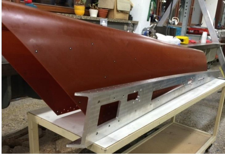
Fig. 4 Manufacturing skin alongside milled aluminium spar.
