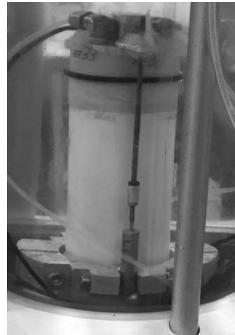
Fig. 2. Chalk sample in triaxial setup.
