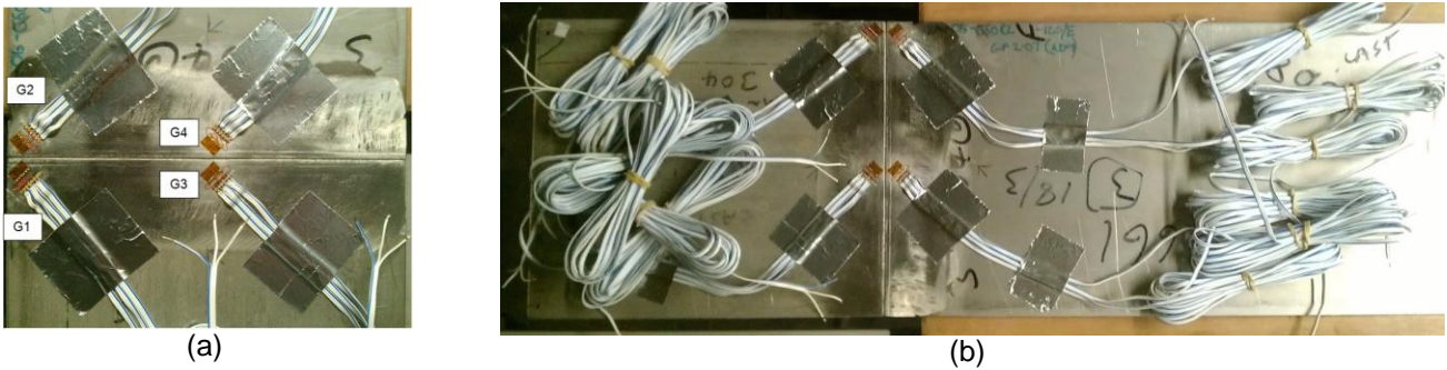
Figure 18 Flange structure equipped with four rosette gages
