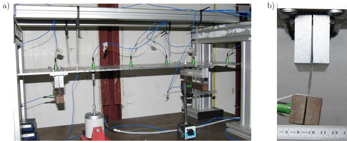
Fig. 1 Test structure representing the configuration of an aircraft wing having two underwing stores supported by pylons. a) General view of the experiment setup. b) Detailed view of the nonlinear connection.
