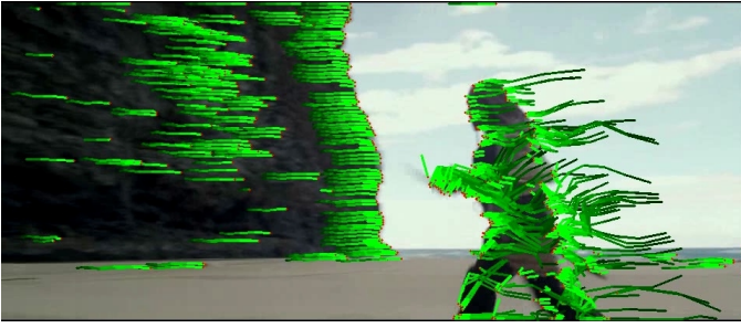
Fig. 6. Monocular dense trajectories detected on a frame from a video depicting the activity “Run”. Red dots show interest point locations in the current frame.
