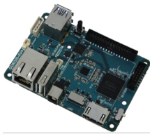
Figure 7: A photo of the Odroid-XU4 taken from the Hardkernel website, alongside the technical specifications of the board.
