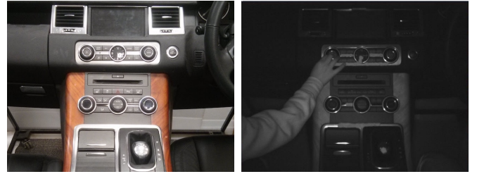
Fig. 1. A control panel: (left) under normal lighting conditions with an RGB camera, (right) with a near infra-red camera with near infra-red illumination.
