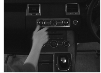
(a) Cabin layout. The camera is mounted on the centre line of the vehicle so its view is not obscured by the front seats.
