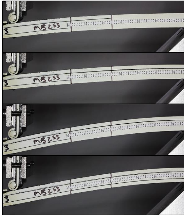
Figure 12 Delamination propagation sequence for control samples (Delaminations highlighted for clarity)
