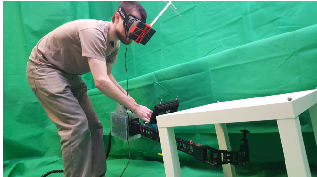
Fig. 1: A cooperative handheld robot assisting a user in a simulated inspection task using a virtual reality headset for feedback.
