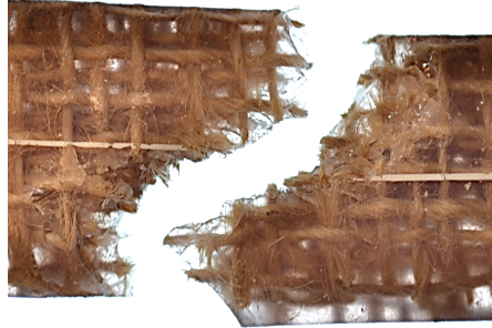
Fig.4 Example of a JFRP sample post torsional static test
