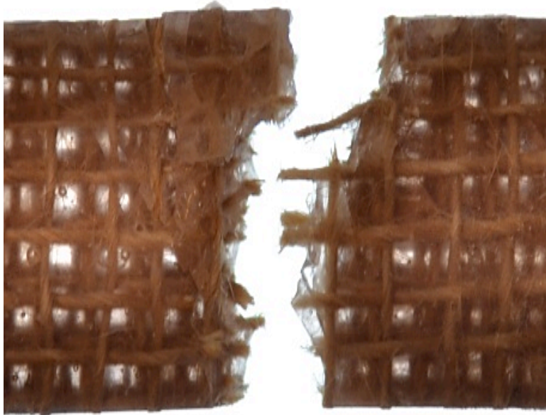
Fig.6 Fracture of a JFRP specimen after the multi-axial static test
