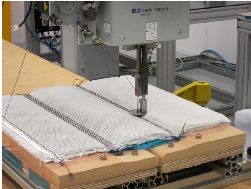
Figure 3: Tufting glass skin-stringer panel with carbon thread
