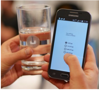
Figure 1: SPLASH allows users to log drinks using NFC-enabled smart-phones to read NFC-tagged cups.
