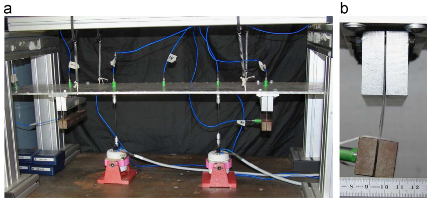
Fig. 10. Test structure representing the configuration of an aircraft wing having two underwing stores supported by pylons. (a) General view of the experimental setup. (b) Close up of the nonlinear connection.
