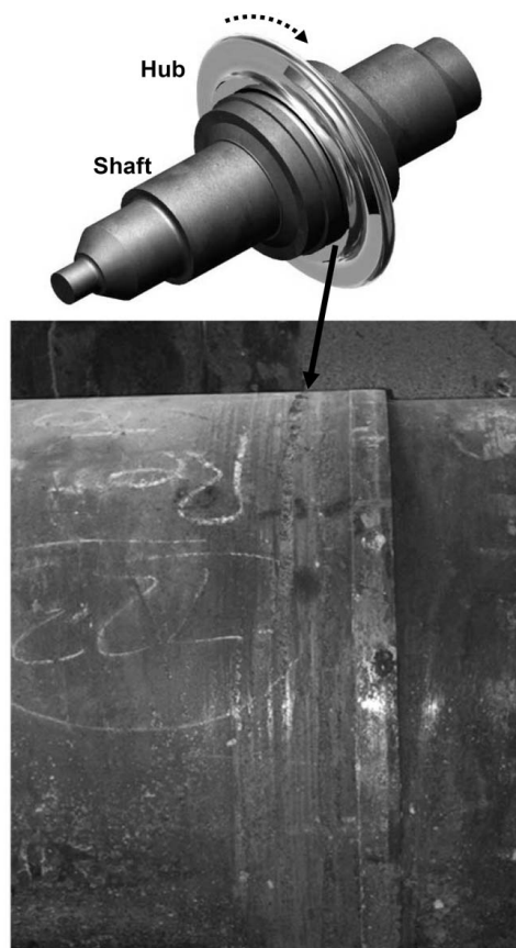
Figure 2 Example of severe ploughing damage on an alloy steel shaft taken from a large hot rolling work roll (diameter ~1000mm)
