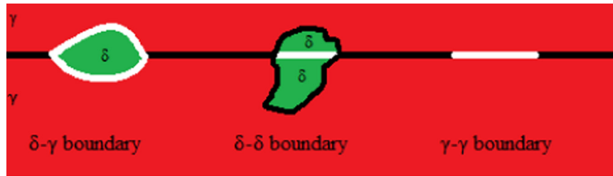
Fig. 12. Schematic showing the three potential locations for cavity nucleation in austenitic steels containing widely dispersed ferrite precipitates. Note that although \delta -ferrite is stated, the ferrite grains in the material may be the evolving low-alloy \alpha -ferrite precipitates. The ferrite–ferrite boundary does not have to be aligned with the austenite–austenite boundary.
