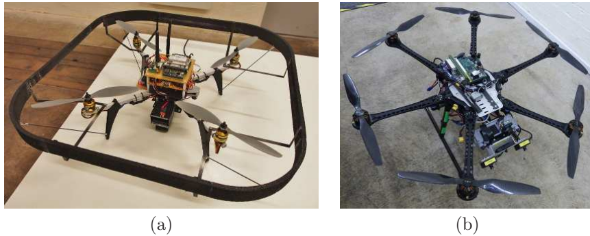
Figure 4: The two aerial vehicles used in this work: (a) quadcopter with an RGB-D camera attached underneath its base, this platform was used to test the auto-retrieval concept; (b) hexacopter platform used in our visual monitoring application, with a monitoring camera on the top and a stereo camera underneath,
