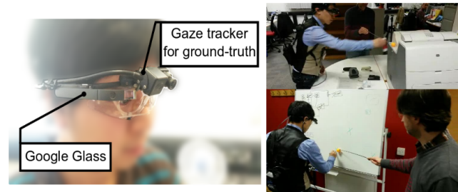
Figure 1: Google Glass and Commercial wearable gaze tracker (for ground-truth) bundle (L) and experimental environment setup (R).
